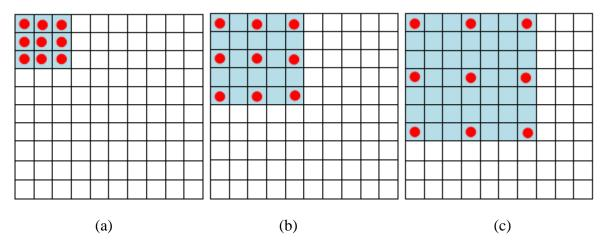
Figure 3. Conceptual illustration of traditional and dilated convolution; (a) traditional convolution (b) dilated convolution with dilation rate 2; (c) dilated convolution with dilation rate 3.
