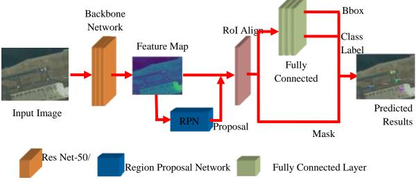
Figure 2. The architecture of Mask R-DCNN object detection
